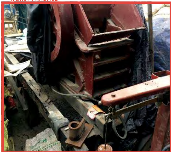
Mill for metals shredding in state of disrepair ©Oeko Institut
