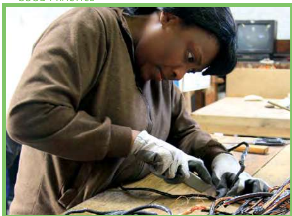
Proper use of equipment to extract copper from cables in South Africa ©Derek Main
