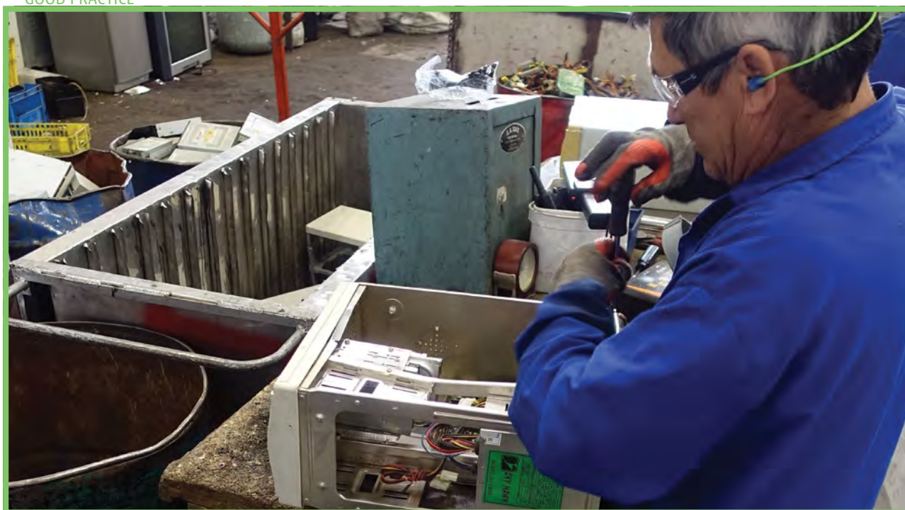
Safe manual dismantling of end-of-life computers to separate materials containing precious metals (e.g. circuit boards) and copper, to be sent to a licensed metallurgical processing facility ©WRF
