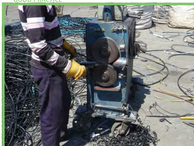
Cable stripper avoiding air pollution (Morocco) ©Empa
