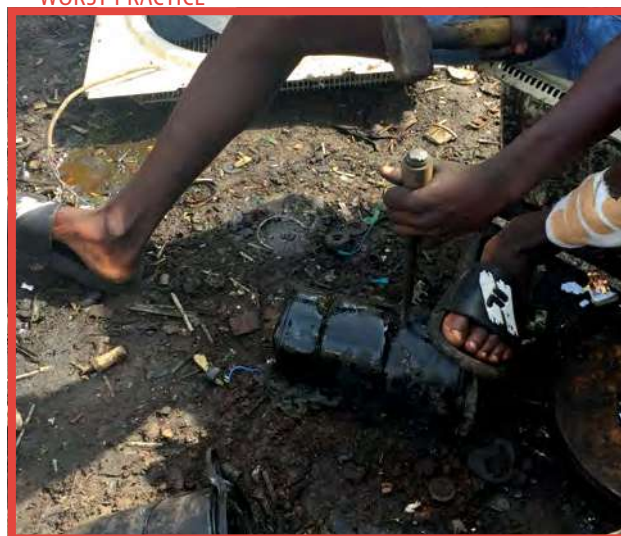
Lubricant leakage from unsafe dismantling of a fridge compressor (Ghana) ©WRF
